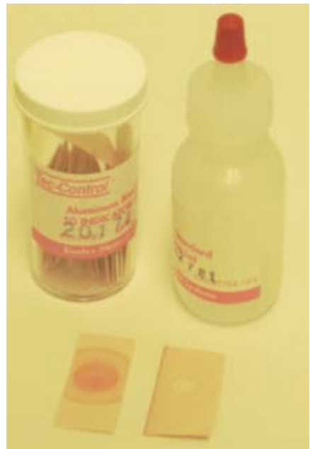
Figure 6: Aluminium breakthrough test (courtesy of VirRAD)
